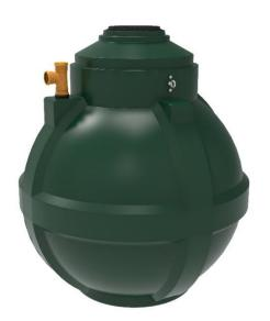
Harlequin's 6000 litre below ground Elsan Waste Tank is designed to safely store caravan toilet waste in a MDPE body compatible with this type of fluid. MDPE tanks are easy to use on site due to the rugged nature of the material. The tank is supplied with lifting eyes as standard for ease of installation. It's designed in accordance with British Standard Code of Practice BS6297 and approved to EN 12566-1 standards.
